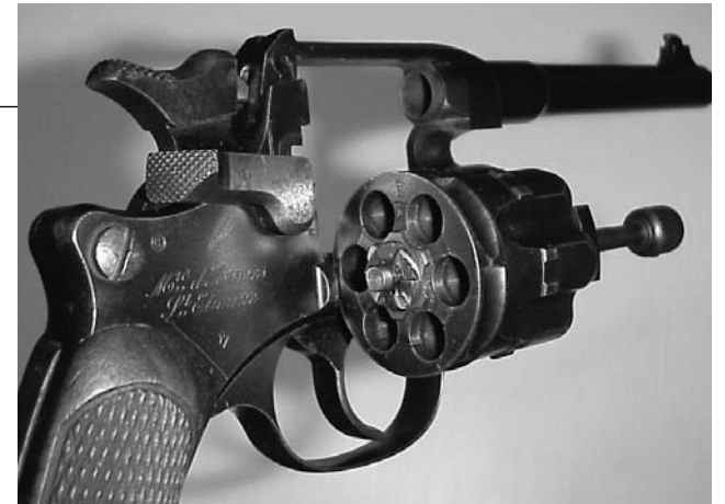
Here's the unique feature of the French Mle 1892 revolver: its swing-out cylinder.
