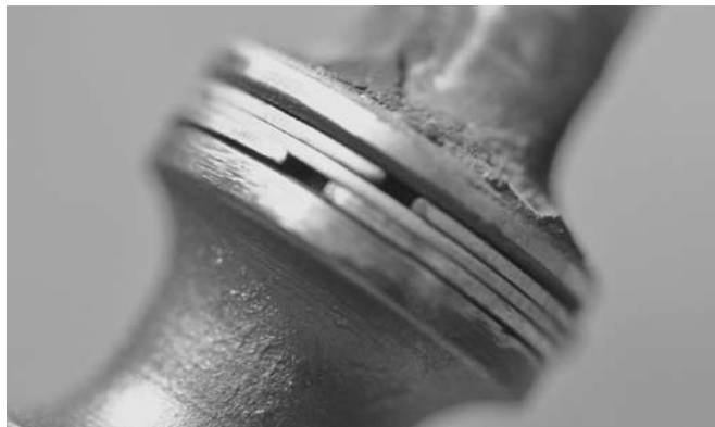
Make sure you have three gas rings, and that the gaps don't line up.
