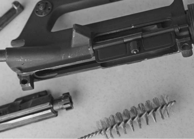
You need a special, big, brush to scrub the interior of the upper.
