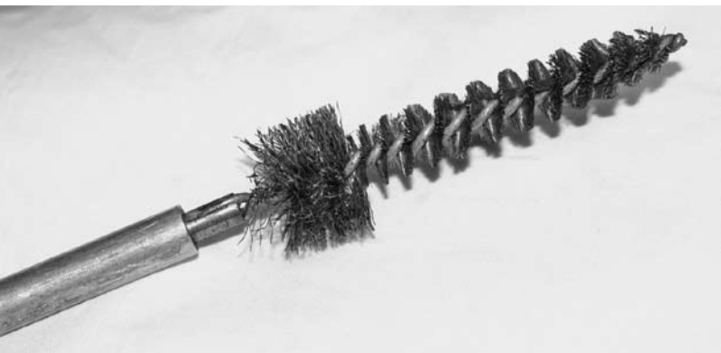
The chamber brush is meant to scrub the chamber and the locking lugs.
