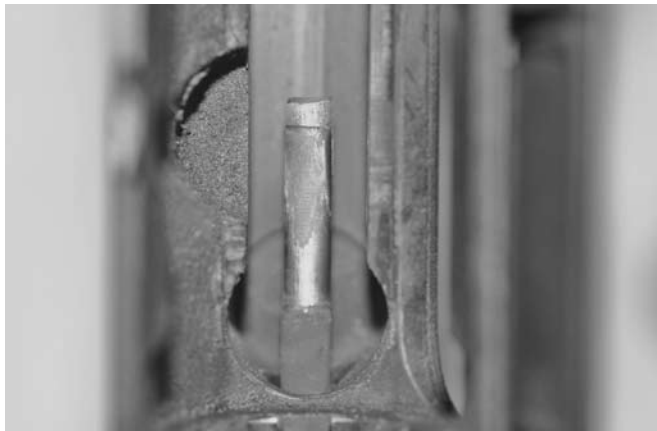
The gas tube blows hot gases into the lubed interior of your rifle.
