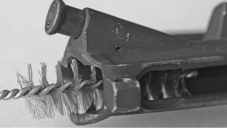
The big brush scrubs the interior, but doesn't get into the charging handle slot. There, you'll need a smaller brush.
