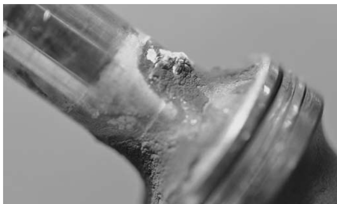
There is a lot of carbon buildup on the bolt tail. Scrape it off carefully, without marring the bolt, or removing gas rings. Don't use a brush.
