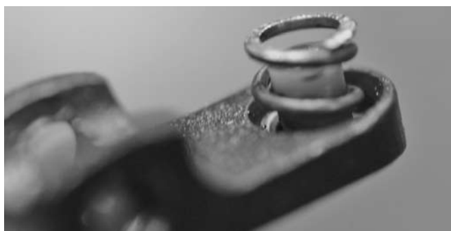
Your extractor should have a blue or black internal buffer. Better yet, add a D-Fender.
