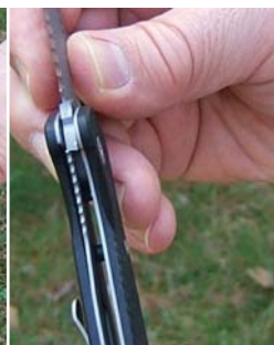
ABOVE: The Ten-Eight is a very useful folder and its pocket clip can be mounted in four different ways; note the holes to receive the mounting hardware
