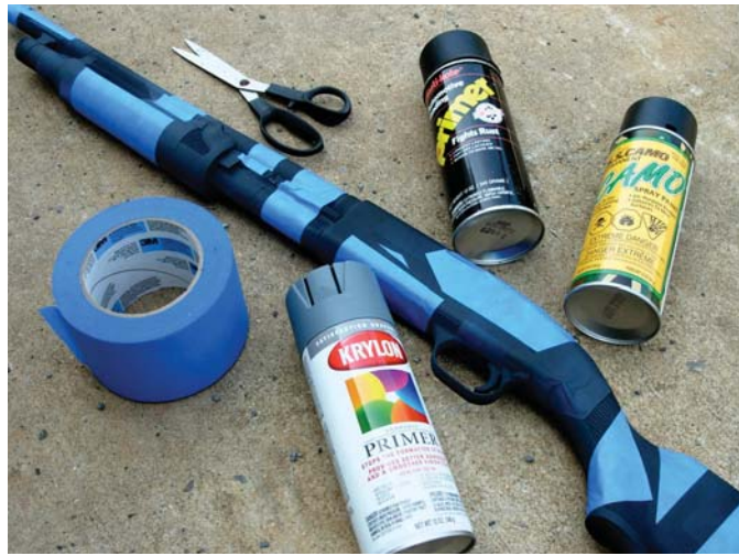
The camouflage process starts by painting the entire gun with flat black primer. The areas that will remain black are covered by masking tape, and then the next color is sprayed. This process is repeated until you've worked in all your colors.
