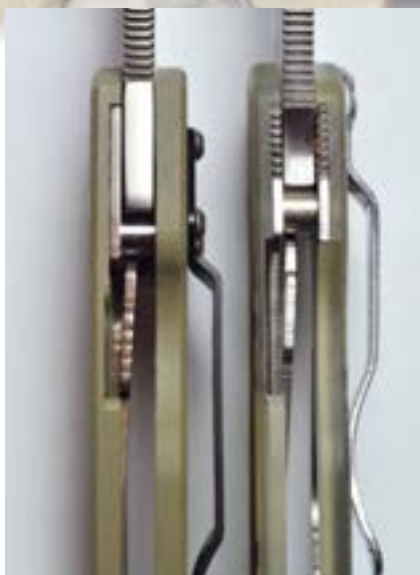
The Compression Lock on the Paramilitary 2 (right) has refined geometry and dimensions compared to the original (left). (David W. Jung photo)
