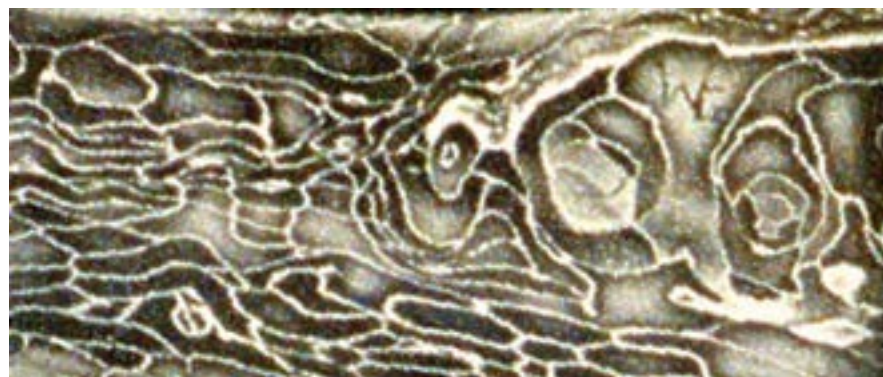
Steel made of wire rope/medium-coarse wires. (Goddard photo)
