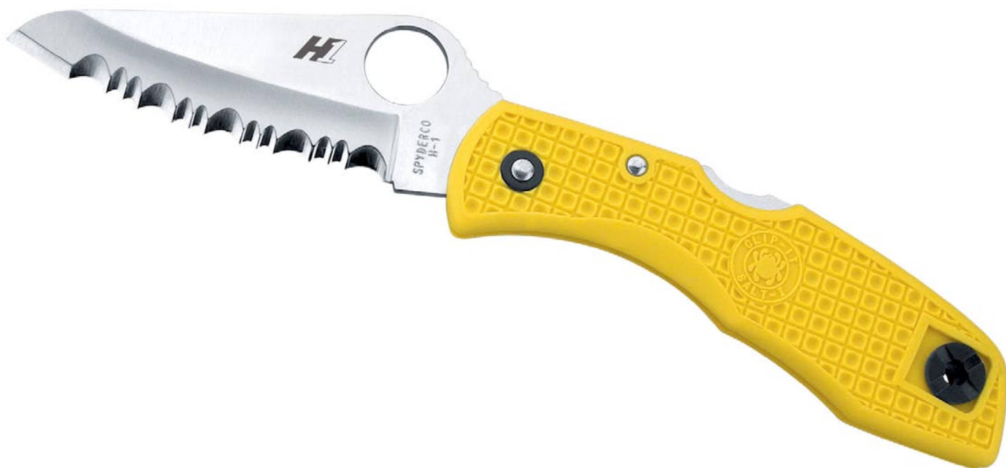
H1 steel comprises the 3-inch blade of the Spyderco Salt I. Closed length: 4 inches. According to the 2011 Spyderco Product Guide, H1 is "entirely rustproof—100 percent. Period." (Spyderco photo)
