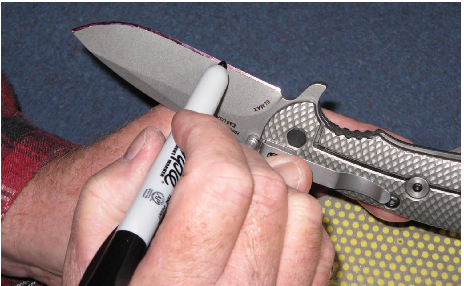
With a black ink Sharpie® permanent marker, color the entire cutting edge or primary bevel on both sides of the blade. The knife is the Zero Tolerance ( www.kershawknives.com/products.php?brand=zt ) Model 0560 flipper folder, a Rick Hinderer ( www.rickhindererknives.com ) design. (Ewing photos)
