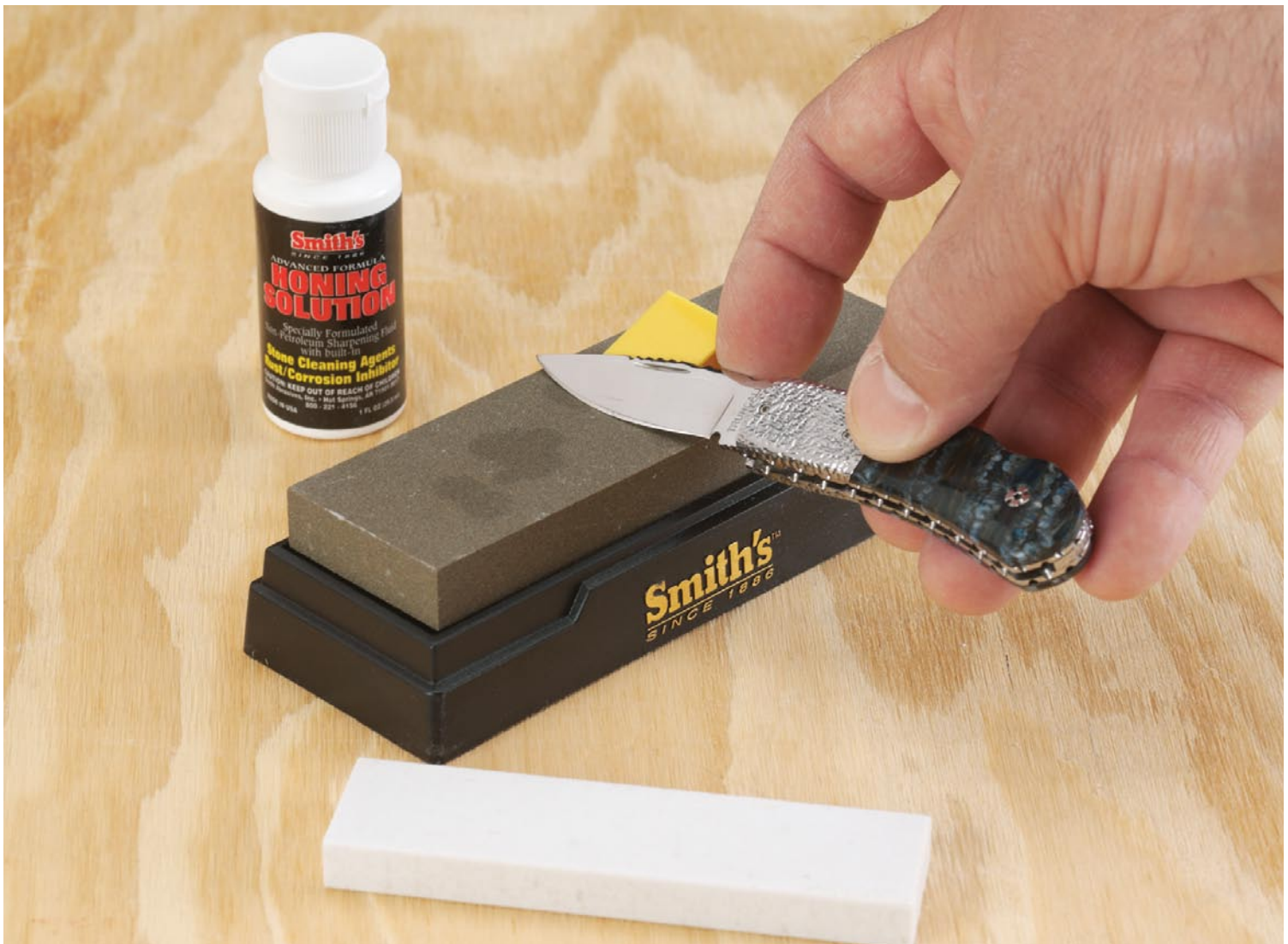
The Smith's 2-Stone Sharpening Kit comes with a small, plastic angle guide that can be placed on the stone. The face of the blade is rested on the guide for the first few times a user hones a blade and until he or she becomes accustomed to holding an angle. The knife is a fileworked Pete Truncali folder.
