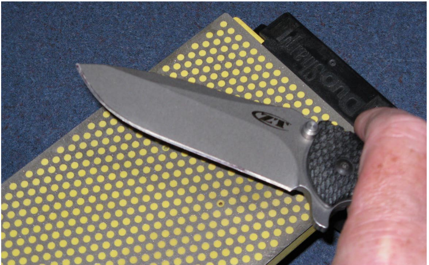
Make a few strokes on the stone (top), doing your best to maintain a consistent angle of blade to hone throughout, and then examine the ink on the edge bevel (bottom). The stone is the DMT DuoSharp, with base. (Ewing photos)
