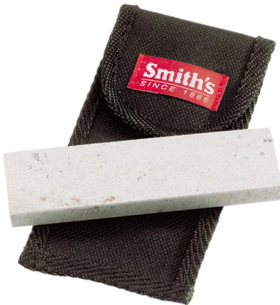
Smith's MP4L sharpens large or small knives with plain edges and also assorted tools. The 4-by-1 3/8-inch medium (soft) Arkansas stone is a 600-grit abrasive. It includes a fabric pouch for storage and protection. (Smith's photo)
