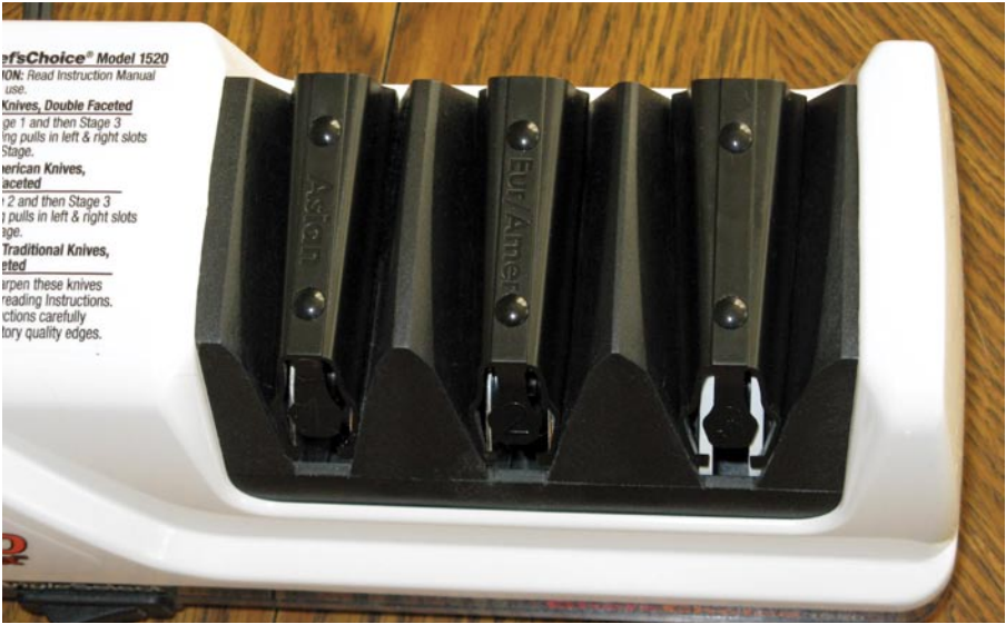
The Chef’s Choice 1520 Angle Select ( http://www.edgecraft.com ) sharpens Asian knives at a 15-degree angle, as well as other common kitchen knives at a 20-degree angle. The left guide of the 1520 is the 15-degree setting for Asian knives, the middle guide (marked “Eur/Amer”) is the 20-degree setting for standard kitchen and sporting knives, and the final guide is for stropping. (photos courtesy of Dexter Ewing)
