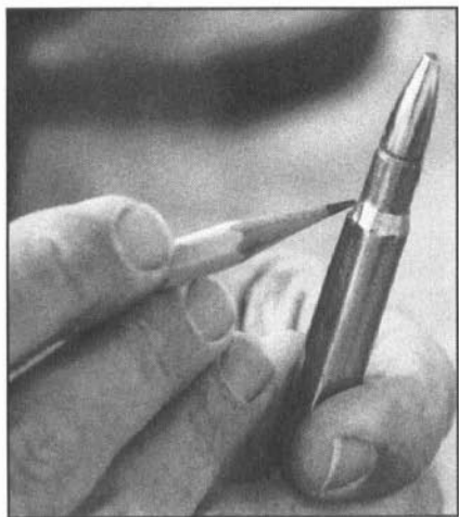
This is the place where the 30-06 case should headspace in an Improved chamber, after creating a shiny ring.
