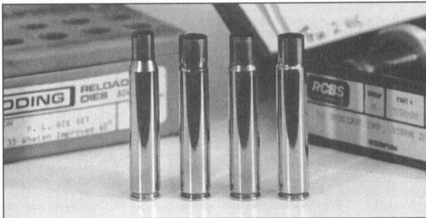
These are the four steps to 35 Whelen Improved: the 30-06 case, the 40-caliber cylinder, the sized case, the fireformed case.
