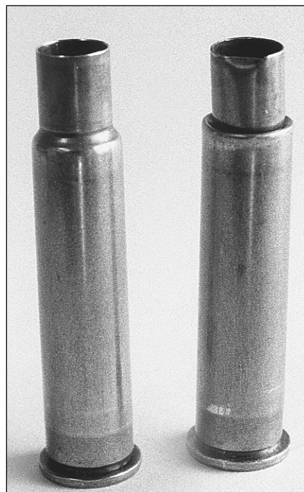
The results of too much force during the loading process. Lack of a gentle touch produced this bent lip and crumpled shoulder on the case at right during bullet seating. Brass used in 30-30 cases is thin, so be careful.
