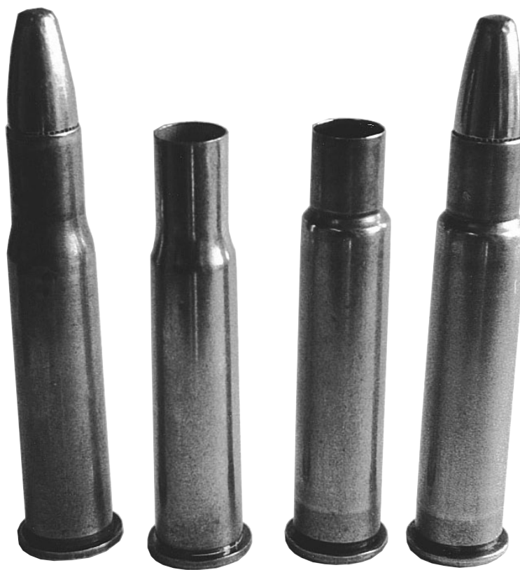
Before and after. Old-timer 30-30 Win. loaded round and case (left) and 30-30 AI conversion. Designed around the turn of the century, the 30-30 Win. has a long neck and gently sloping shoulder and sides that contribute to case stretch and eventual head separation. The more modern 30-30 AI has straight-sided case walls and sharp 40-degree shoulder, making it more suitable for reloading.
