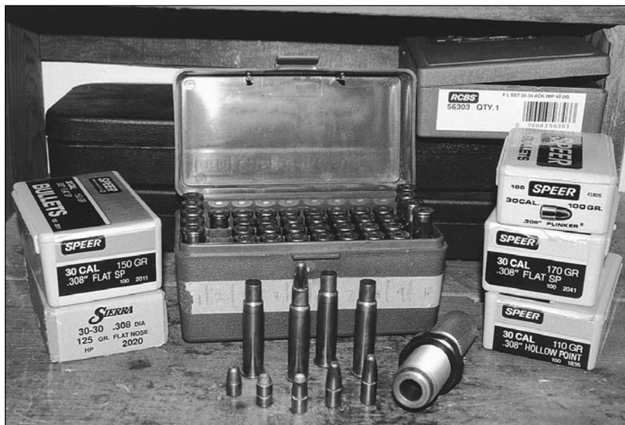
Some of the components and dies used for reloading the 30-30 AI. More modern design makes for longer case life and less case stretch while giving higher velocities.
